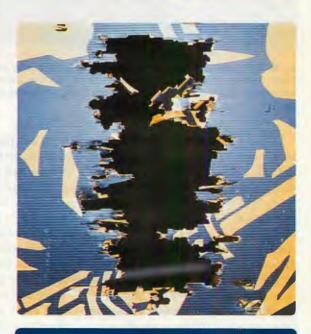
This target was on the receiving end of a 540-round burst from the Mk5 pod weapon, plus a full payload each from the single- and triple-barreled guns. As the .22LR AM 180 submachine gun demonstrated, a very high rate of sustained fire can damage a target completely out of proportion to the caliber and weight of the rounds fired. Metal Storm similarly emphasizes the structural damage potential of its systems, even firing at "only" 45,000 rpm.
